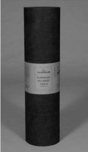
**Product Use:** Flintglas® Ply 4 is designed for use as a base and/or an inter ply for hot applied, built-up roofing systems and hybrid modified bitumen systems. It is suitable for use in the construction of various types of membranes for both new construction and reroofing over a variety of substrates. It is specially constructed to provide uniform strength and promote improved asphalt uniformity and adhesion between plies.
